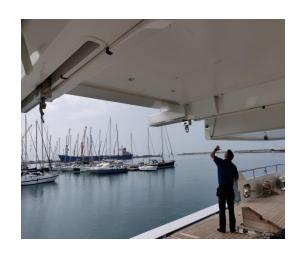
The list of equipment which falls within this definition is long and varied, and will include everything from chain blocks to fixed lifting points, davits, deck cranes and more. In addition to lifting appliances, lifting tackle (or loose gear) needs the same level of inspection. This is defined as any type of equipment that is suspended below the hook, such as a shackle or sling.
